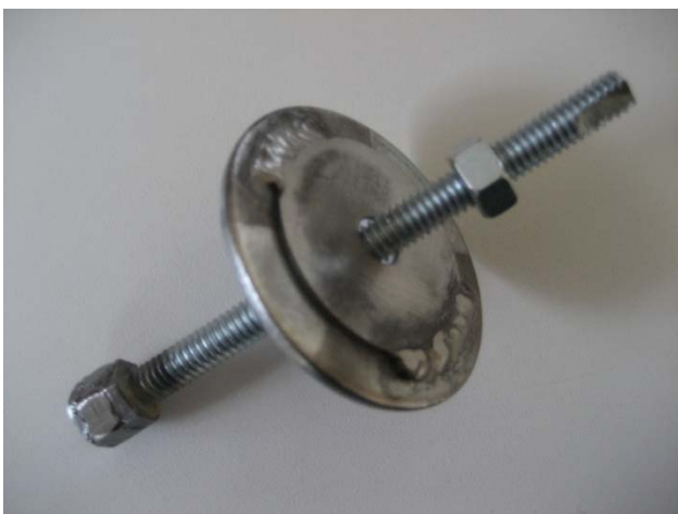
Picture 3 A homemade grease cup extractor tool
