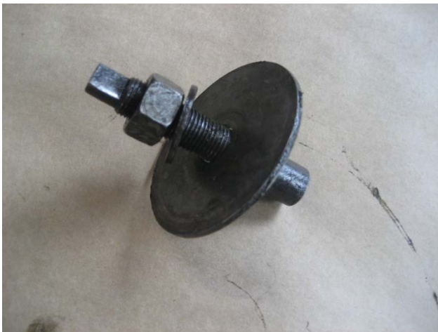
Picture 3 A homemade grease cup extractor tool
