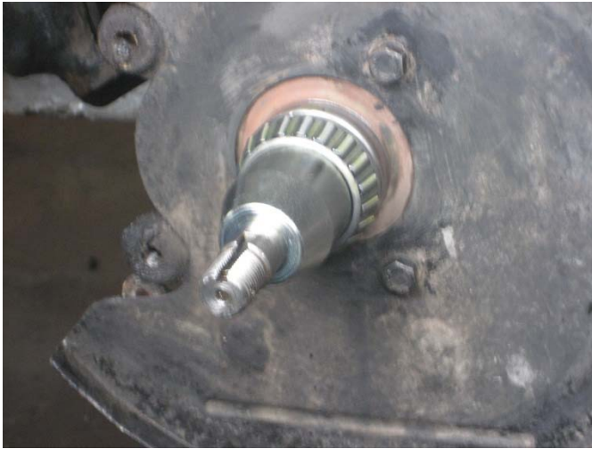
Picture 5 Looking inside the hub showing where a drift can be used to drive out the old races (at 3 and 9 o'clock)
