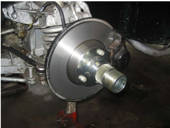
Picture 6 The finished hub and disc assembly. (A new hub and disc was used in this install).
